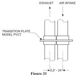
In both vertical and horizontal colinear direct vent applications, a colinear transition plate model PVCT can be used to minimize clearances between intake and exhaust pipes.
